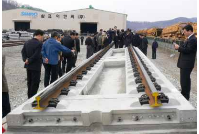
PSTS Frame at the SAMPYO factory
